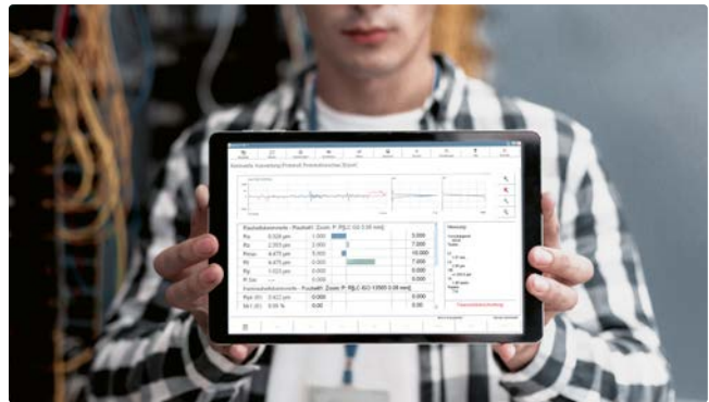
"RoughnessPlus" section: Virtual rulers to interactively set distances in X and Z direction in the profile field
